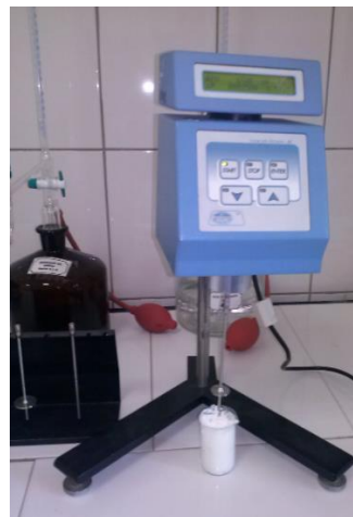
Fig.2 ViscoStar R Viscosimeter
